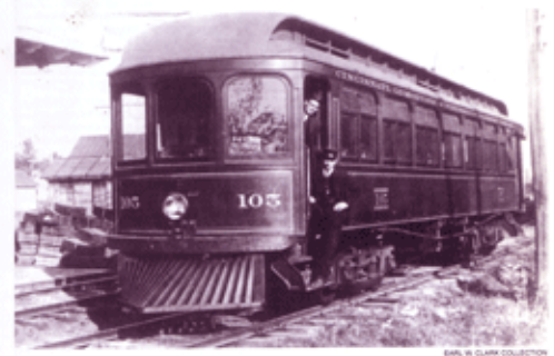
The image of the classic midwest interurban, typified by car No. 105 of the Cincinnati, Georgetown & Portsmouth Railroad. No. 105 was built by St. Louis Car Co. in 1902, as part of a series of ten cars, numbered from 100 to 109 by ST. But this electric railroad was more than an "interurban," as it had narrow-gauge tracks and a steam railroad tradition. Car 101 stayed on the CG&P until the 1935 abandonment.
